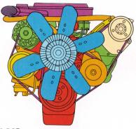
**305 V8.** Our 305-cubic-inch engine with a 2-barrel carburetor is available on all models, except in California where the 350-4 V8 is required. Features of our 305 V8 that contribute to responsive performance include a short stroke to reduce friction, valve-in-head design for free breathing, precision-balanced crankshaft, full-jacket cylinder cooling.
